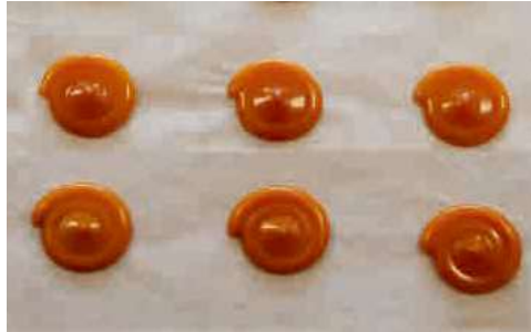
Mixing result eco-DUOMIX (dynamic mixing) 混合结果 eco-DUOMIX(动态混合)
