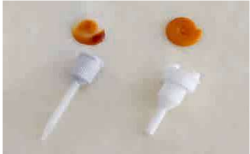
Comparison: Mixing result static mixing (left), mixing result dynamic mixing (right)
